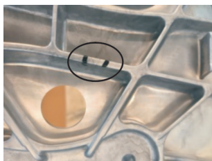
图19 加强筋冷隔 Fig.19 Cold shut in the reinforcing rib
