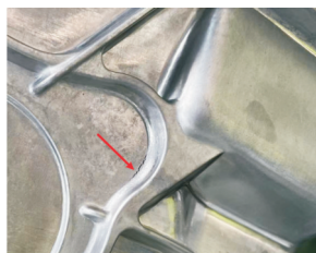
图20 R角裂纹 Fig.20 R-angle crack
